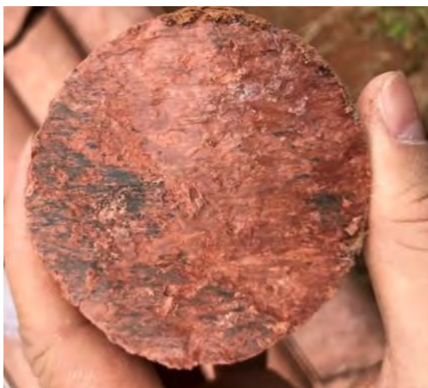
Figure 2 – Slip zone core of Landslide No. 2
