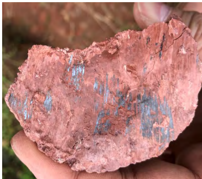
Figure 3 – Slip zone core exhibiting slickensides
