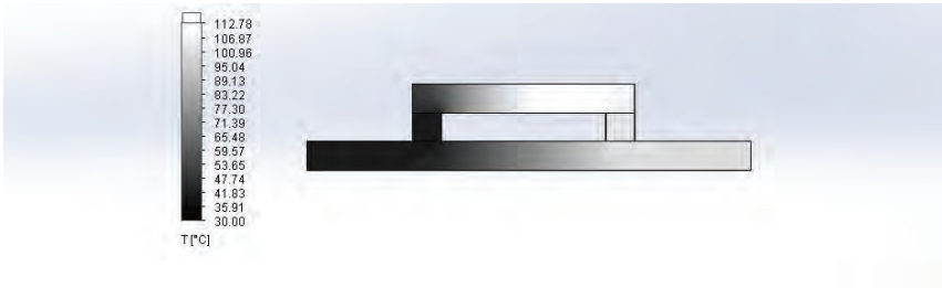
Figure 4. The thermal model of configuration of interconnect metal lines Figure 1 (a) with a non-uniform temperature profile
