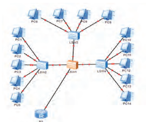
Fig. 2. Logical topology and VLAN segmentation of the designed corporate network
